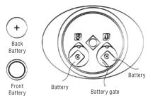
The picture below illustrates the correct way to change the batteries. Rotate the lower cover anticlockwise to open. Remove the batteries with a rod-like object, and insert the new batteries. Then place the cover back onto the base, and rotate clockwise to lock and close the lower cover.
