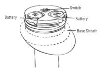
Take precautions to ensure that the batteries are placed in the correct position.
